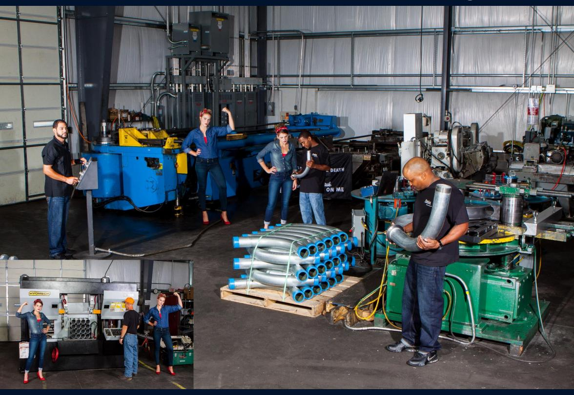
Patriot loves large scale projects. Our large diameter and large radius Wallace Bender takes about 30 seconds to bend a 6" Standard 90. Our 5 Unit Pedrick Bending Workcell is comprised of Two D15 Benders and Three A7 Benders. Visit us in Virginia if you'd like to see some of the fastest and most accurate benders in the industry.
